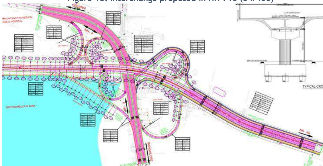
Figure 14: Interchange proposed in NH 48 (km 76/900)
